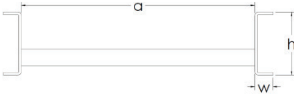
Figure 8: Cable ladder cross-section with basic dimensions
