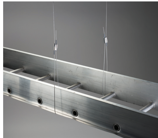
Figure 10: Speed Link SLK supporting a wire basket tray (left) and a cable ladder (right) This could also be completed using the infinite loop application where the wire is looped around the structure and the load and attached to itself in one location.
