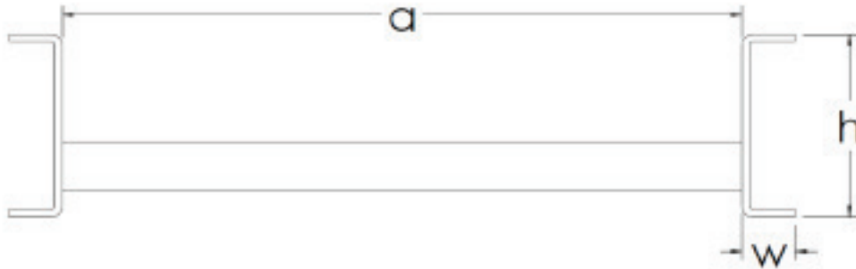
Figure 2: Cable ladder cross-section with basic dimensions
