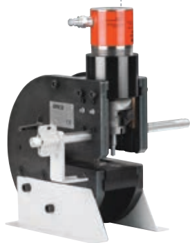
硬铜排及柔性母排液压冲孔机
