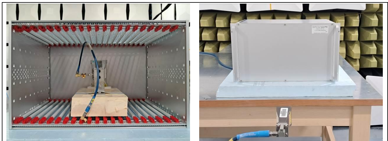
Figure 6-16: test setup horizontal, 18 – 40 GHz
