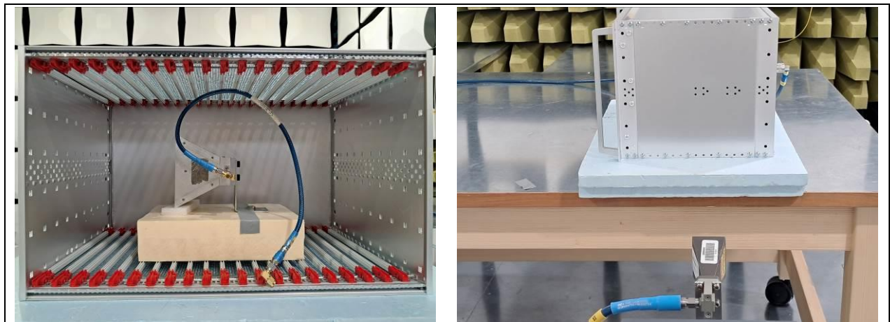
Figure 6-18: test setup horizontal, 18 – 40 GHz
