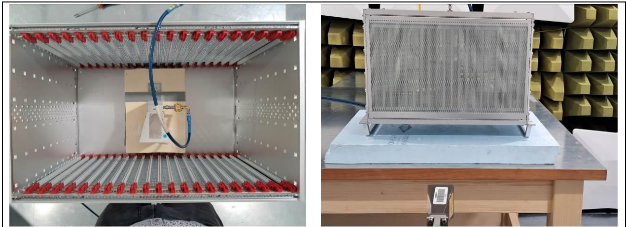
Figure 6-20: test setup horizontal, 18 – 40 GHz
